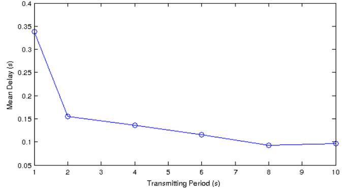
Fig. 10. Mean end-to-end delay retransmissions from the Switch node. The delay significantly grows with transmission periods below 2s, as the duration of the contention period increases with the workload.
