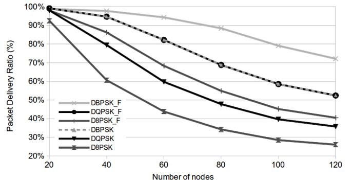
Fig. 6. Packet delivery ratio vs. the number of nodes.
