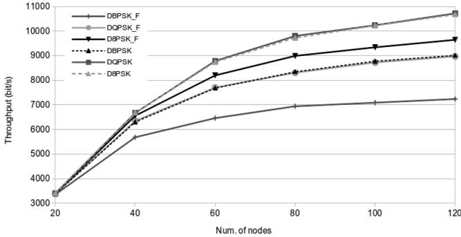
Fig. 5. Throughput vs. the number of nodes.
