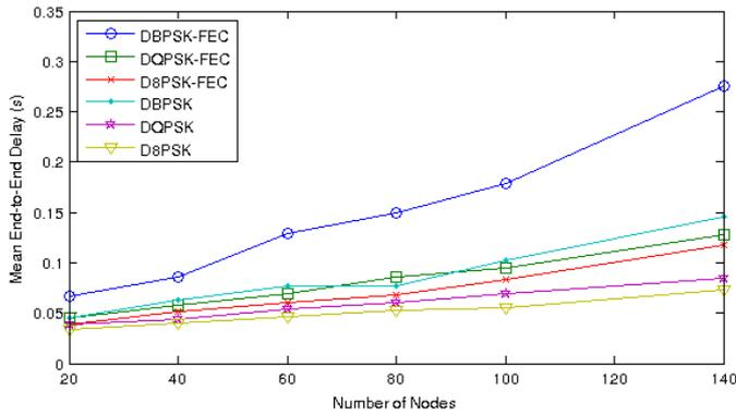
Fig. 8. End-to-End delay vs. the number of nodes.
