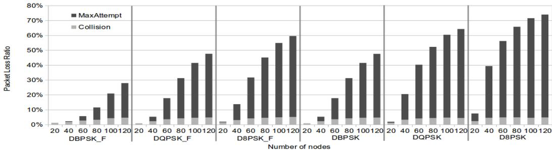
Fig. 7. Packet Loss Ratio (for each modulation scheme) vs. the number of nodes.
